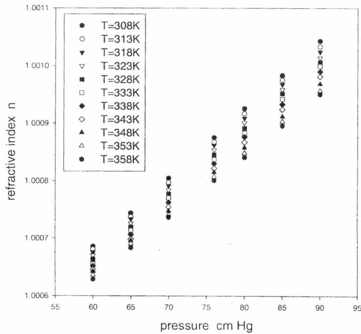
Fig. 4b. An example of pressure dependence of refractive index at constant temperature and laser wavelength, for Freon<sub>12</sub>,  $(dn/dp)_{T,\lambda}$ .
