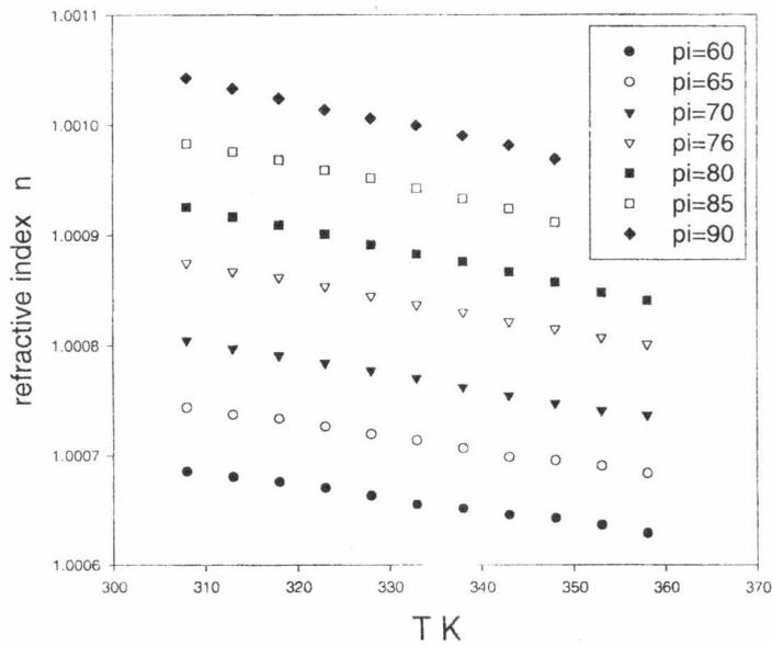
Fig. 5b. An example of temperature dependence of refractive index at constant pressure and laser wavelength, for Freon<sub>12</sub>,  $(dn/dT)_{p,\lambda}$ .
