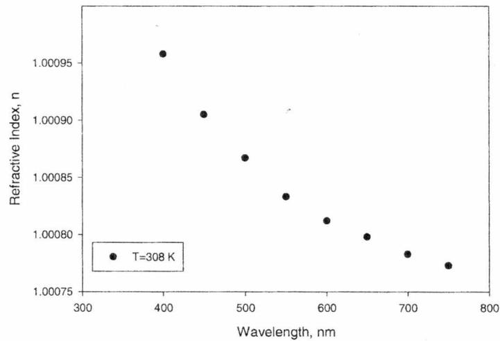
Fig. 3b. Wavelength dependence of refractive index for Freon<sub>12</sub> at constant temperature and pressure,  $(dn/d\lambda)_{p,T}$ .
