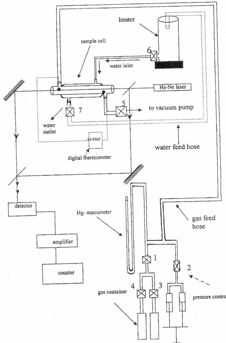
Fig. 1. The constructed set-up used for measuring the gas's refractive index.
