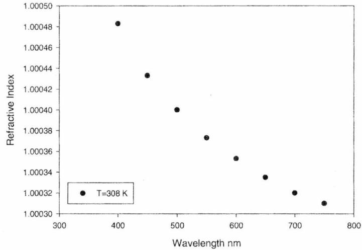
Fig. 3a. Wavelength dependence of refractive index for Carbon dioxide at constant temperature and pressure,  $(dn/d\lambda)_{p,T}$ .
