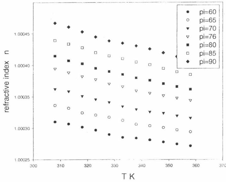
Fig. 5a. An example of temperature dependence of refractive index at constant pressure and laser wavelength, for Carbon dioxide,  $(dn/dT)_{p,\lambda}$ .
