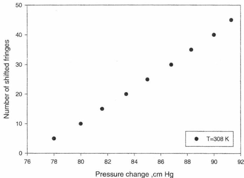
Fig. 2. An example of determination of gas's refractive index as a function of gas's pressure at constant temperature by using the constructed MZIS of Carbon dioxide gas.
