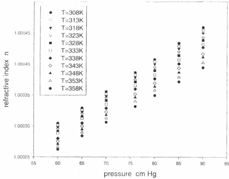
Fig. 4a. An example of pressure dependence of refractive index at constant temperature and laser wavelength, for Carbon dioxide,  $(dn/dp)_{T,\lambda}$ .
